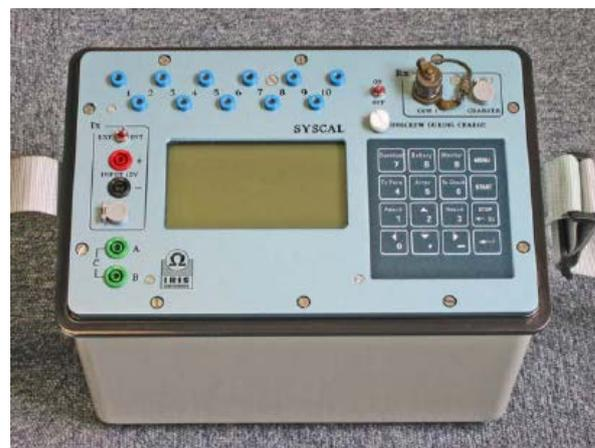
Figura 9 – Georesistivimetro Syscal PRO (Geostudi Astier srl, 2008).
