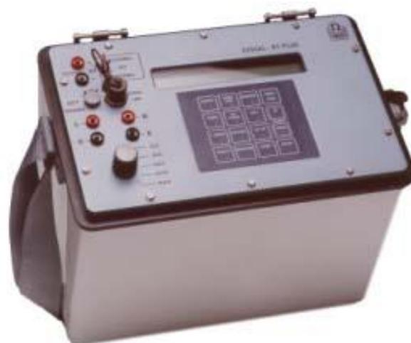
**Figura 8** – Georesistivometro Syscal R1 Plus (fonte: <http://www.resistivity-meters.com/>).
